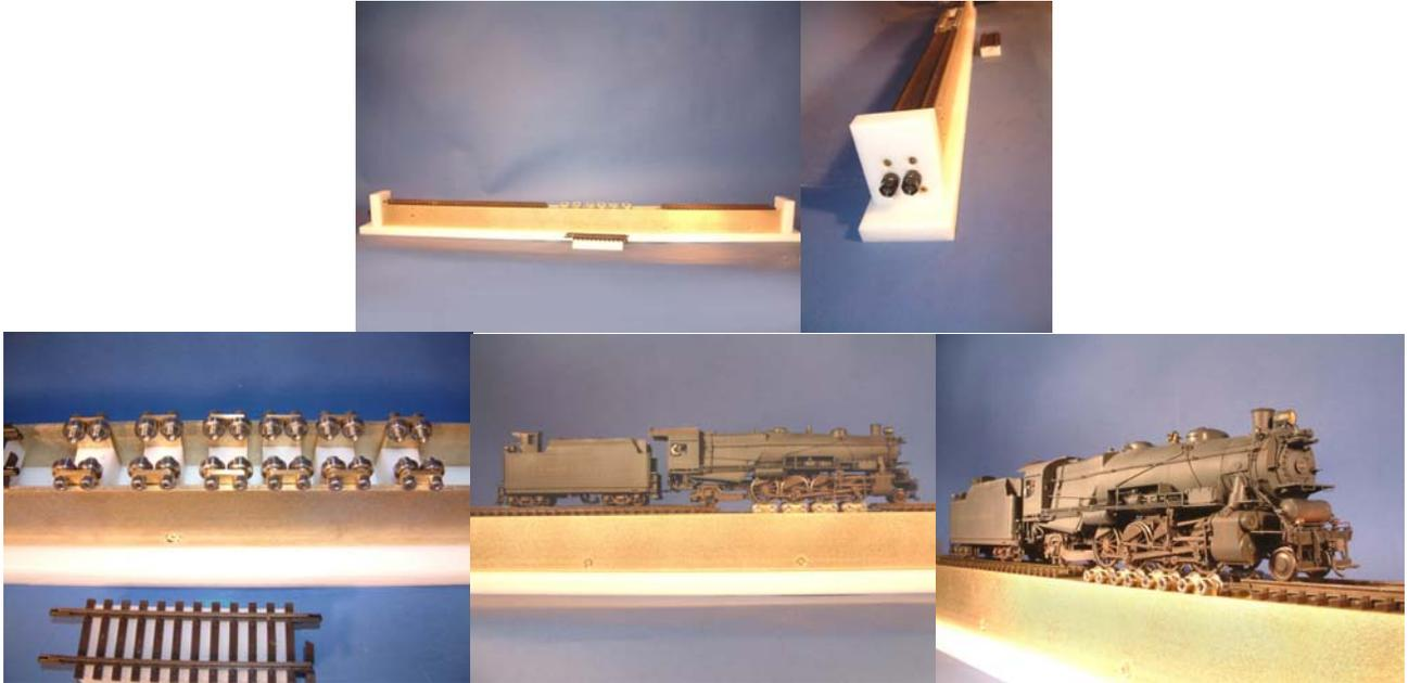
This roller test track will accommodate American Flyer and Scale locomotives. Use it to demonstrate a locomotive at a train show, program a DCC and sound unit, or look for a short. All of the track sections are removable except the 4' piece at the terminal end. It can be reconfigured to run 2 small locomotives at the same time with the available 2 extra roller sets, all the way up to a big 4-8-8-4 articulate. It is over 3 feet long and is completely American made!
